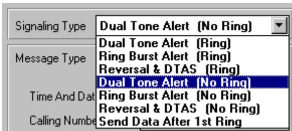
The list of available signaling options depends on the selected standard, and the state of the CPE's hook switch. If the CPE is on-hook, then only the Type I signaling options will be shown. In the case of an off-hook CPE, then the Type II options are displayed.
