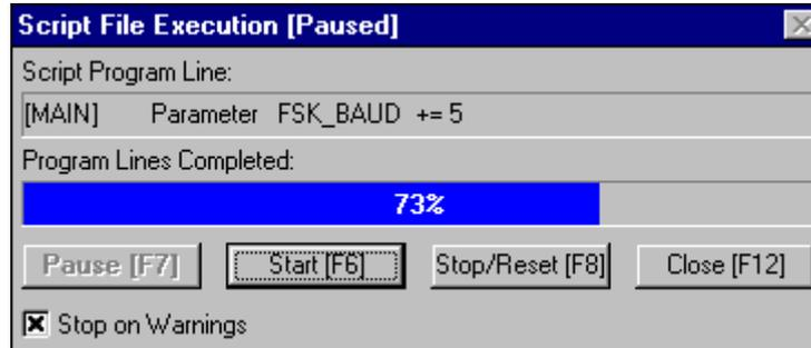
The Script Execution window shows the current script program line being processed, along with a scale showing percentage of program lines completed. This scale is only accurate assuming that no branches have been taken during the execution of the script program.
