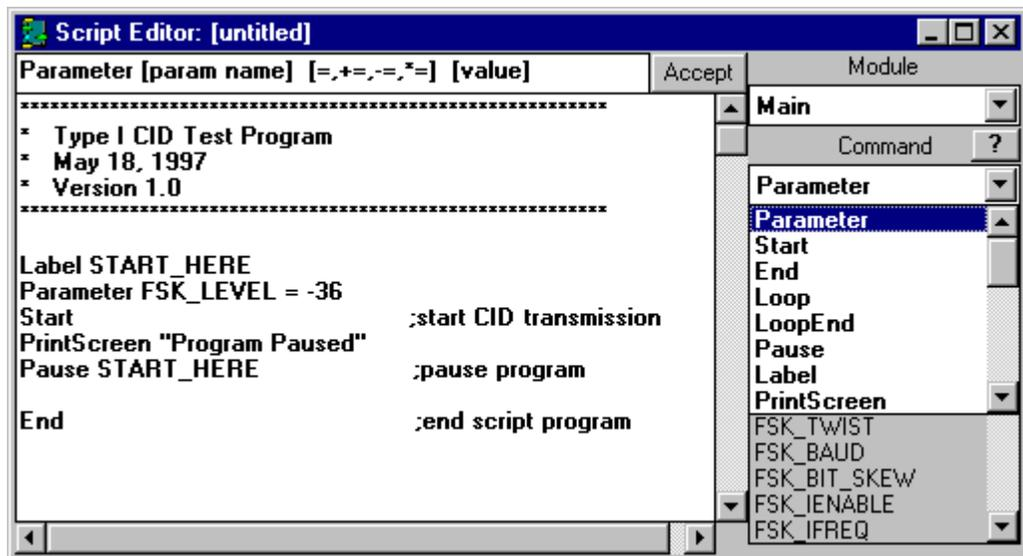
To enter the parameter name, scroll the list box until you find the parameter you wish to modify. Double click on this parameter. The parameter name will be transferred to the composing text line. Now the list box fills with further options for the parameter. As before double clicking on the item in
