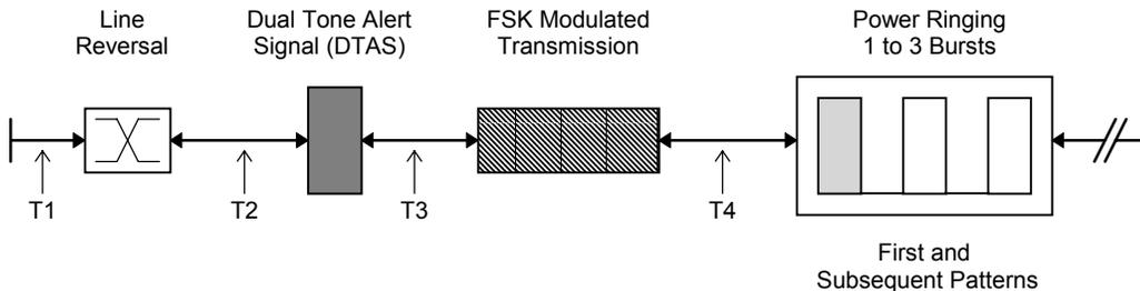
T1 is the time delay before the reversal of the telephone line, while T2 is the time interval between the line reversal and the generation of the DTAS tone. The interval between the DTAS and the FSK data is defined by T3. If ringing has been enabled, then T4 specifies the delay between the FSK data and the start of ringing.
