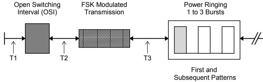
The time interval T1 represents the beginning of the Caller ID transmission and the generation of the OSI. The length of the OSI can be set to any arbitrary time interval. Following the OSI, is interval T2 which precedes the FSK data transmission. Once the FSK data has been sent T3 defines the time to ringing, provided it has been enabled. The parameter category, name, and default value for each of these parameters is as follows:
