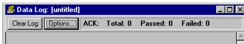
Every time a Type II Caller ID transmission is started, the ACK Total count is incremented by one. Depending on the received ACK tone, either the Passed or Failed count is incremented. The timing, level, and frequency criteria governing the ACK tone reception is controlled by the parameters in the Advanced Setup window.
