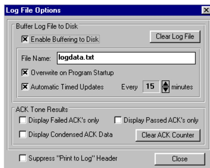
The Log File Options control panel defines if and how the data log will be buffered to a disk file and the display format for Type II Caller ID transmission. Since the data log window will only display the
