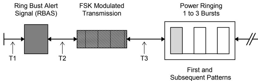
The time interval T1 represents the beginning of the Caller ID transmission and the generation of the RBAS tone. The length, frequency, and level of the RBAS tone is independently set. Following the RBAS, is interval T2 which precedes the FSK data transmission. Once the FSK data has been sent T3 defines the time to ringing. The parameter category, name, and default value for each of these parameters is as follows:
