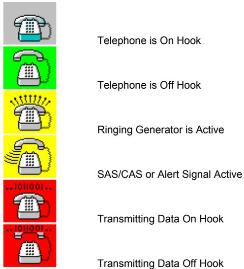
If the telephone is in an on hook state, the current line voltage is displayed to the left of the status icon. Likewise, if the telephone is in an off hook state, the loop current is displayed to the left of the status icon.
