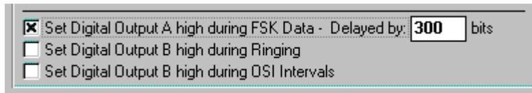
By clicking the mouse at the appropriate check box above, the output A or B will output a high level when that event is active. This feature can be useful in triggering external equipment such as oscilloscopes, logic analyzers, and emulators during key times of the Caller ID transmission.
