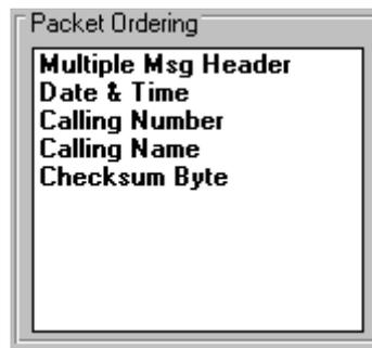
The transmission order of the packets is from the top to the bottom. In this case the Multiple Msg. Header (which contains the Message Type and Message Length bytes) is the first packet to be transmitted. Following this is the Date & Time, Calling Number, and Calling Name packets. The last packet is called the Checksum Byte which contains a single byte that represents the checksum of all the packets listed.
