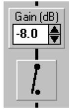
To enable the signal mixer, click the mouse on the graphical switch. This will toggle the state of the signal mixer between on and off. The mixing gain can be adjusted using the up and down spin controls, or by entering a numeric value. The default state for the mixer is off, and upon restoring program defaults, or changing operational standards, the mixer will be turned off.
