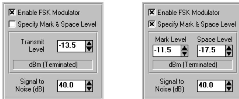
At anytime the total FSK transmit level is changed, the mark and space tone levels are re-calculated to reflect the new total level and maintaining the existing twist level. If the FSK twist setting is changed, the mark and space tone levels are re-calculated to reflect the new twist settings and maintaining the existing total level setting.
