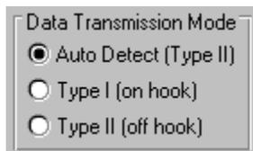
The Type I mode refers to Caller ID transmissions with the telephone in the on hook state, and usually accompanied with power ringing. Type II mode refers to Caller ID with Call Waiting (CIDCW) operation, with the telephone in the off hook state. If the Auto Detect mode has been enabled, the operational mode will change depending on the current state of the hook switch. If on hook, Type I Caller ID transmissions will be sent. If off hook, Type II (CIDCW) transmissions will be sent.
