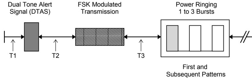
The time interval T1 represents the beginning of the Caller ID transmission and the generation of the DTAS tone. The length of the DTAS tone is independently set. Following the DTAS, is the interval T2 which precedes the FSK data transmission. Once the FSK data has been sent T3 defines the time to ringing, provided it has been enabled. The parameter category, name, and default value for each of these parameters is as follows:
