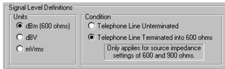
The units of dBm specify that all signals will have their level defined relative to 1 milliwatt of power into a 600 ohm load. The dBV unit specifies levels relative to 1 Vrms, while the unit of mVrms is self-explanatory. Irrespective of what units the levels are specified in, they can refer to a telephone line terminated into 600 ohms, or an unterminated telephone line.
