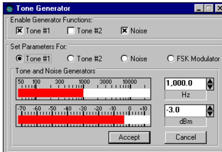
To change the settings of either tone #1, tone #2, or the noise generator, click the button associated with that tone or noise signal in the "Set Parameters For:" section of the window.
