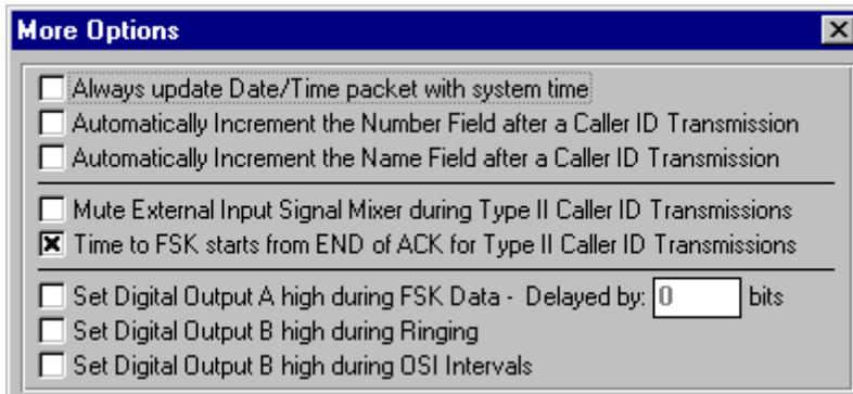
The More Options window can be viewed by selecting the [CONFIGURATION] [MORE OPTIONS] menu command, or by pressing the CTRL-Z key combination. The default setting is enabled.
