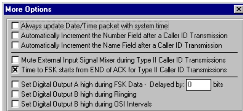
The forth option "Mute External Input Signal Mixer during Type II Caller ID Transmissions", controls the behavior of the signal mixer during Type II transmission. The external input signal mixer will allow the user to combine the signal present at the external input BNC connector, with the tones and
