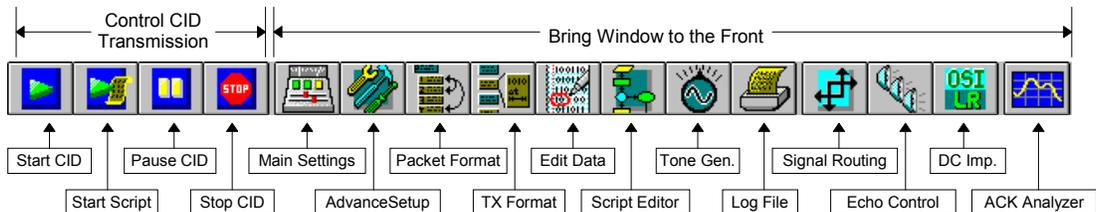
The first four buttons control the transmission of the Caller ID data. Pressing the START button, launches a Caller ID transmission. PAUSE will suspend its state indefinitely, while STOP will terminate it. START SCRIPT will start the execution of scripting programs, which help to automate complex test sequences.
