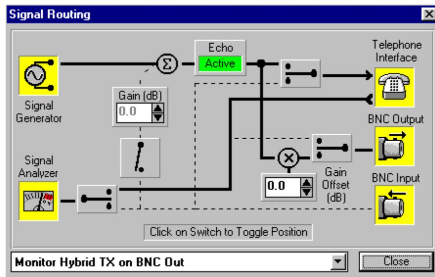
By changing the signal flow, the BNC connectors can be used to monitor the transmit or receive signal to and from the telephone. Or to provide for a loop through configuration for the transmit or receive path where externally applied signals or filtering can be added to the signals being generated by the TSPC or analyzed by the TSPC. The BNC connectors can also be configured so that the user has direct control over the signals being sent to and from the telephone interface.
