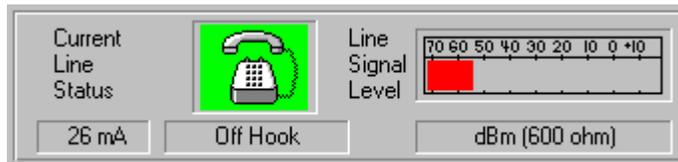
The telephone icons display various states or conditions experienced by the telephone under test. All of the possible telephone icons are shown below:
