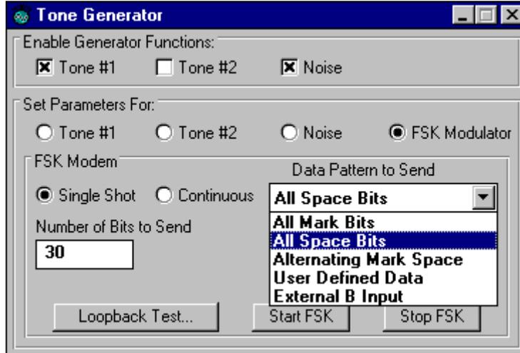
For loop back testing, the FSK modulator is expected to generate an alternating mark/space bit pattern. If this is not the selected data pattern selected for the FSK modulator, a warning message will be displayed when clicking the "Loop back Test" button. The alternating mark/space pattern will be read by the Com Port as an ASCII character 'U'. If any other character is received by the Com Port, it is treated as an error, and will be displayed.
