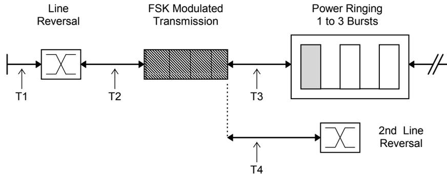
T1 is the time delay before the reversal of the telephone line, while T2 is the time interval between the line reversal and the FSK data. If ringing has been enabled, then T3 specifies the delay between the FSK data and the start of ringing. Otherwise, a second line reversal occurs at a time interval T4 after the FSK data has been sent.
