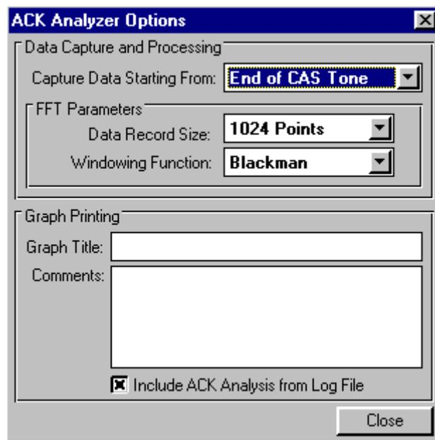
In addition to the data capture and FFT processing options, a graph title and comment can be entered. These two fields will be printed along with the waveform displayed, by selecting the [FILE] [PRINT ACK ANALYSIS WINDOW] menu command. If the check box labeled "Include ACK Analysis
