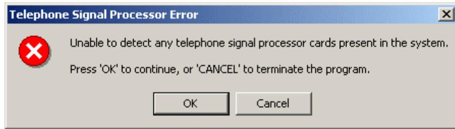
The CID1500 must be configured to search for an AI-7280 instead of a TSPC at start up. To change the setting, click the 'OK' button for the above message and then select the [HARDWARE SETUP] command from the [CONFIGURATION] menu. This displays the following window, from which the CID1500 software can be told which hardware device to use.
