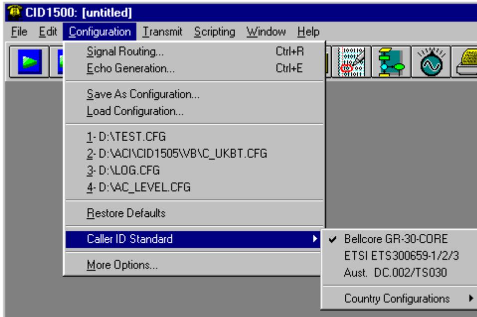
Changing the standard is simply accomplished by selecting the Caller ID Standard option under the Configuration menu, as shown above. The three different standards that can currently be selected are Bellcore GR-30-CORE, ETSI (European Telecommunications Standards Institute) ETS 300659-1/2/3, and the Australian Caller ID System based upon DC.002 and TS 030 (1997).
