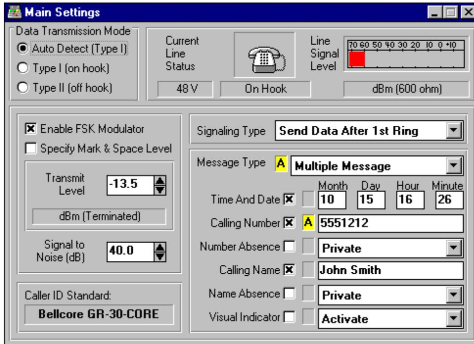
The key areas of the Main Settings sub-window are the Data Transmission Mode, Line Status, and CID Transmission Parameters.
