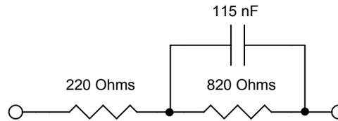
Figure 2. ZR Impedance
