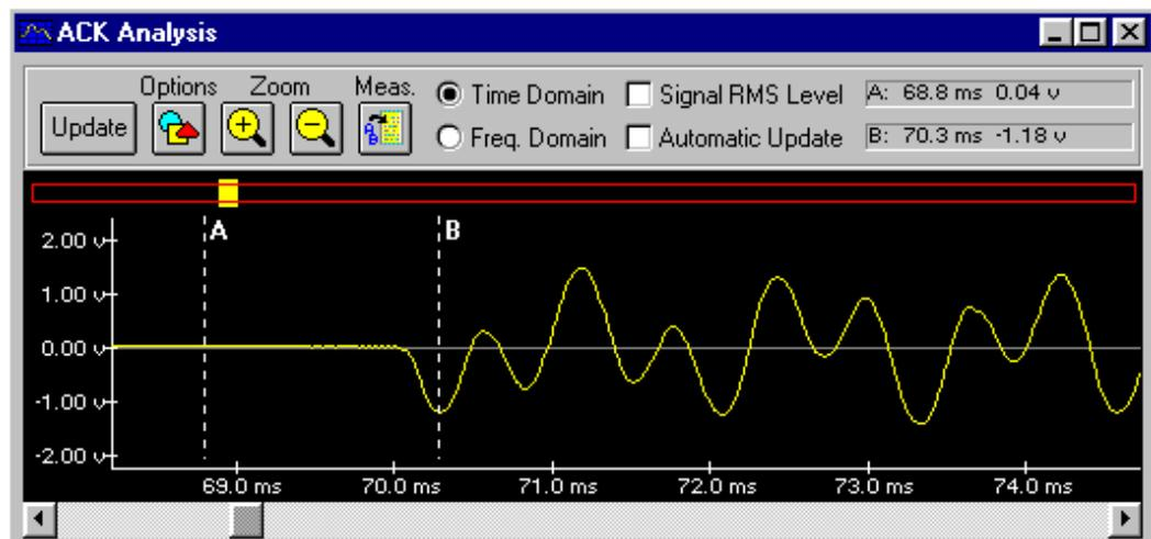
The time domain view can also show the captured data in terms of its RMS signal level. This is done by enabling the check box labeled Signal RMS Level on the ACK Analyzer window. If this check box is enabled, the vertical axis of the time domain view will represent the RMS signal level of the captured data.
