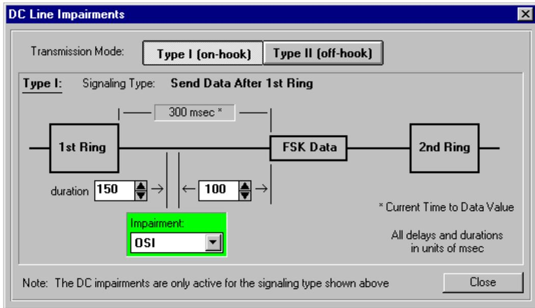
A graphic diagram is used to simplify the timing relationship between the various parameters for both the Type I (on-hook) and Type II (off-hook) cases. The two Transmission Mode buttons, at the top center of the window, control whether the Type I or Type II conditions are displayed.
