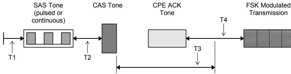
Figure B: Time delay to FSK data referenced to end of ACK
