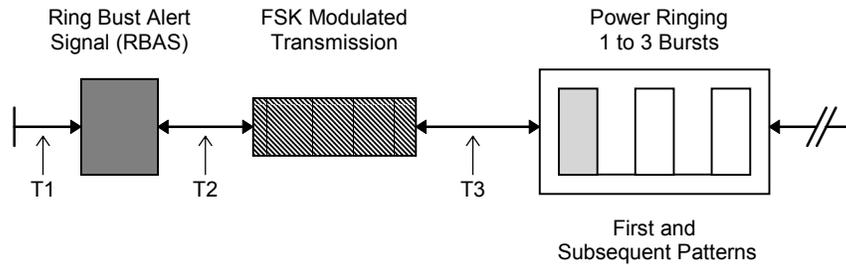
The time interval T1 represents the beginning of the Caller ID transmission and the generation of the RBAS tone. The length of the RBAS tone is independently set. Following the RBAS, is interval T2 which precedes the FSK data transmission. Once the FSK data has been sent T3 defines the time to ringing, provided it has been enabled. The parameter category, name, and default value for each of these parameters is as follows:
