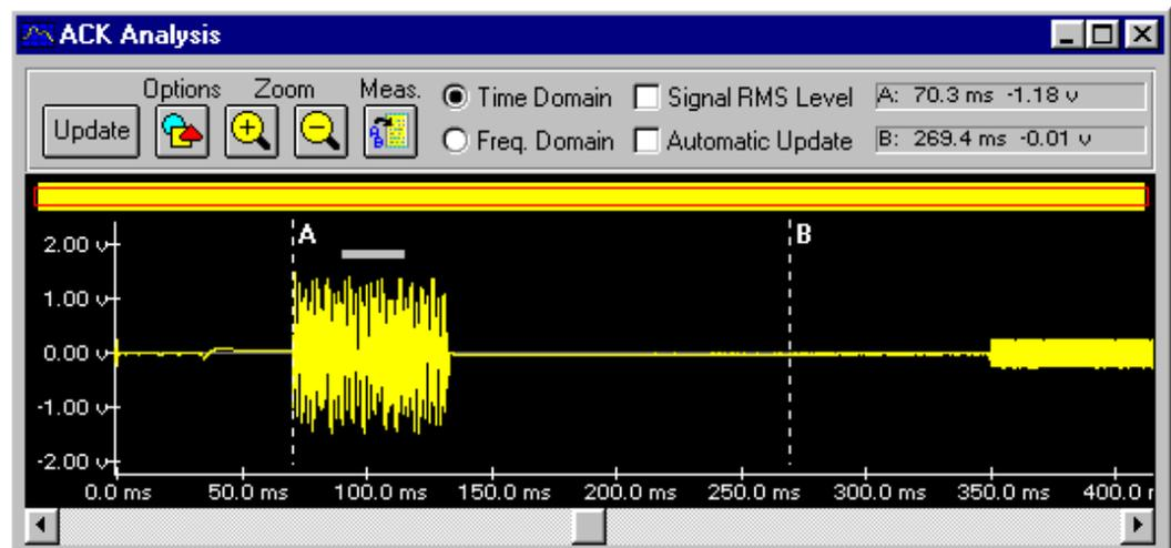
In the example shown above, an ACK tone from a CPE was captured and is displayed in its full span. In this case the ACK tone was generated 70 msec after the end of the CAS/DTAS tone. A small transient signal can be seen to be generated by the CPE at a time of 40 msec. The lower level signal starting at a time index of 350 msec is the beginning portion of the FSK data being transmitted to the CPE.
