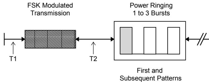
The time interval T1 represents the beginning of the Caller ID transmission and the start of the FSK data transmission. If ringing has been enabled, then following the time interval T2, the ring generator will be started. The parameter category, name, and default value for each of these parameters is as follows:
