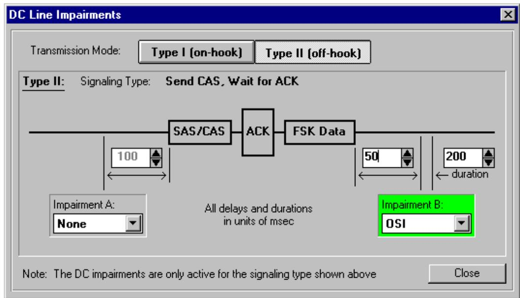
In this case, two independent impairments can be selected to occur before the SAS and CAS tones and after the FSK data transmission. As with the Type I, settings, the impairment is selected from the drop-down list box, and can be either an OSI, line reversal, or none.
