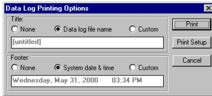
In addition, a script program can change the printing options via the LOG command. Any changes made to the settings are stored within a configuration file.
